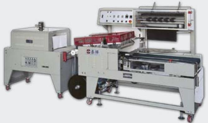
One example of Tayi Yeh's development efforts is the SA-106-2 Fully Automatic Counting & Collating Single Layer Colorful Film Packaging Machine, which is available in both sleeve type and double line models.
