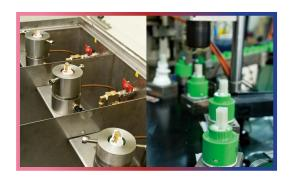
The ceramic cartridges use uni-block plastic injection parts for consistent quality, and are assembled via automation for standardization. Each item has to pass stringent quality control and pre-shipment tests to assure zero defect, including tests for air-pressure leakage, cycle, breaking, high temperature, high pressure, and intermittent impact.
