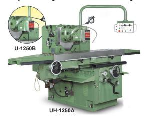
iron in three axes with two or four slideways and are capable of doing stable and high-efficiency precision machining.
