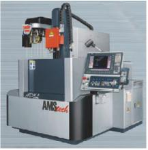
various manufacturers, while the invert spindle reduces electrode wear and improves accuracy of drilling, and various canned cycles as the CHMER and edge find can be used throughout drilling.
