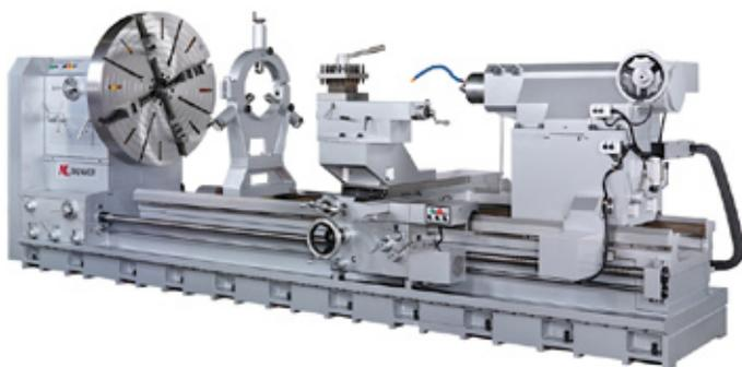
In addition to these families of machines, the company has developed heavy-duty precision CNC facing lathes featuring a middle-mounted Z-axis ballscrew.
