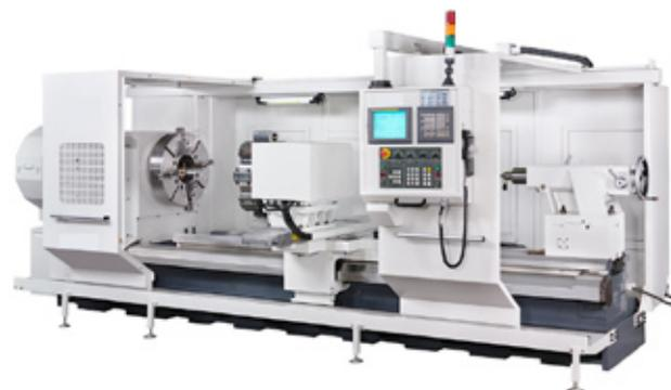
The company is currently promoting its HL, HK, DHL, DHK and RHL series of heavy-duty lathes, which are laden with useful features. They have spindle bores that range from 6, 9, 10, 12 and 15 inches in diameter and working beds that come in widths of 24 inches, 32 inches and 49 inches. Their swing-over beds range from 960mm, 1,120mm, and 1,220mm to 2,000mm in diameter, and distance between centers 1,500mm-8,000mm in the Z axis.
