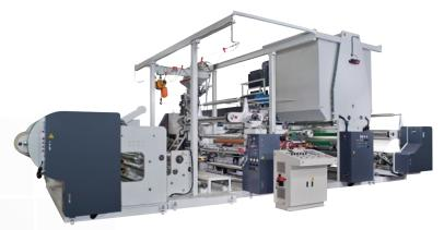
by setting the desired speed, when the series are used to produce products with different coating thickness. The series can also satisfy end-users with paper coating 10 micron in thickness.
