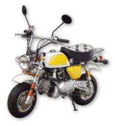
Song Ying utilizes low-pressure electronic fuel injection designed inhouse to achieve eco-friendliness and cost efficiency. A kick starter is included for manual start-up in case of low battery, and an error sensor provides for immediate troubleshooting on the road. The firm's creed is that constant innovation is key to competitiveness and sustainability.
