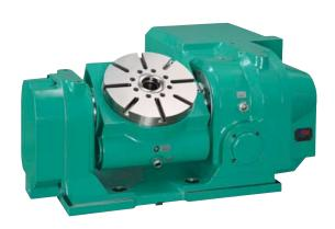
The company's TRT-series of CNC tilting rotary tables features a two-axis motor driver with dual lead worm transmission, 0.001 continuous increment operation, a hydraulic clamping system (PHC booster available), and a wider tilting angle for improved operation. Its NCT-series of CNC rotary tables works in both vertical and horizontal positions.
