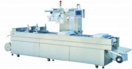
Thermoforming machine AVM-425
