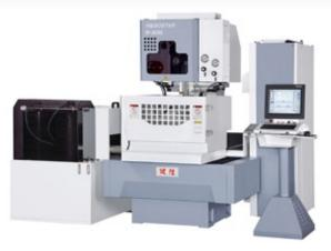
interface, outstanding control system, PCD-specific (polycrystalline diamond) micro-wire electric circuit, high-rigidity spindle, high-accuracy linear guide-way, automatic wire-threading system etc.
